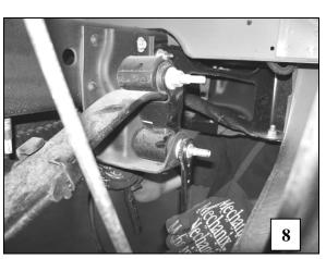
Remove bracket and reverse center bolt
