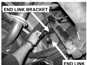
**STEP 3B:** The simplest way to install the new Anti-Sway Bar is by mounting the ends of the Sway Bar to the ends of the end links. Begin by attaching one end at a time. Using an adjustable jack stand to help in supporting the Anti-Sway Bar, hold one end up to the end link and insert the mounting hardware. Do this to both ends.
