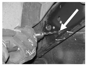
**STEP 1F:** With the END LINK BRACKET off the chassis tube frame and the three holes drilled out to 3/8", insert the nut-serts supplied with the kit (there should be a total of 10 in the kit) (See Parts List). With the nut-sert, nut sleeve and bolt assembled, push the nut-sert into the holes, making sure they are flush to the chassis tube frame.
