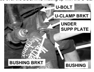
**STEP 3G:** Using a 9/16 wrench or a ratchet with a 9/16 socket head, tighten and lock down the mounting hardware.
