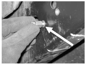
**STEP 1G:** To lock the nut-sert in place in the chassis tube frame, using a 7/16" wrench or a ratchet with a 7/16 socket head (bolt) and a 1/2 wrench (nut sleeve), begin tightening the bolt. The knurl end of the nut-sert locks into the thickness of the chassis tube frame, while the end expands on the inside. Tighten until you are not able to turn it anymore, just stopping short of not being able to turning it. Do this for all three holes that have been just drilled.
