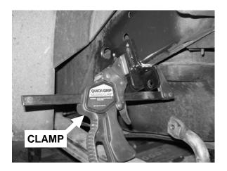
**STEP 1D:** Using a 9/32 drill bit, and with the END LINK BRACKET clamped in place, drill the three (3) clearance holes into the chassis tube frame.
