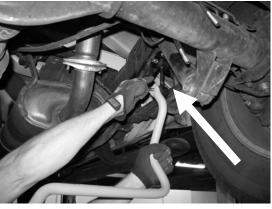
**STEP 3C:** Tighten both hardware to torque specs.
