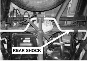
**STEP 3F:** Slide the U-shape mount screw over the top of the rear axle, with the legs pointing downward. The U-CLAMP bracket will face up with the legs facing upwards. The UNDER SUPPORT PLATE will locate between the UNDER SUPPORT PLATE and the back of the BUSHING. The BUSHING BRACKET will slide over the BUSHING mating up with the U-CLAMP.
