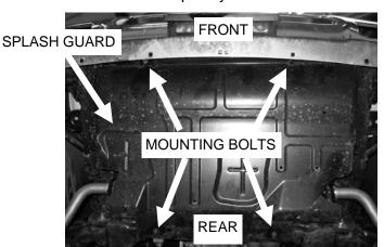
**B.** Using a 10mm wrench, or an air ratchet with a 10mm socket head, remove all four screws.
