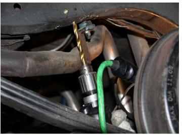
**5.** You must follow the installation instructions for kit No. 5501 attached when installing these brackets. Holes must be drilled in the correct place. Failure to do this will result in the miss alignment of the bracket.
