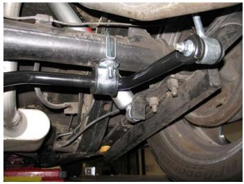
**4.** Using an existing hole on both side of the frame, measure 2 3/8" from edge of hole to edge of bracket.
