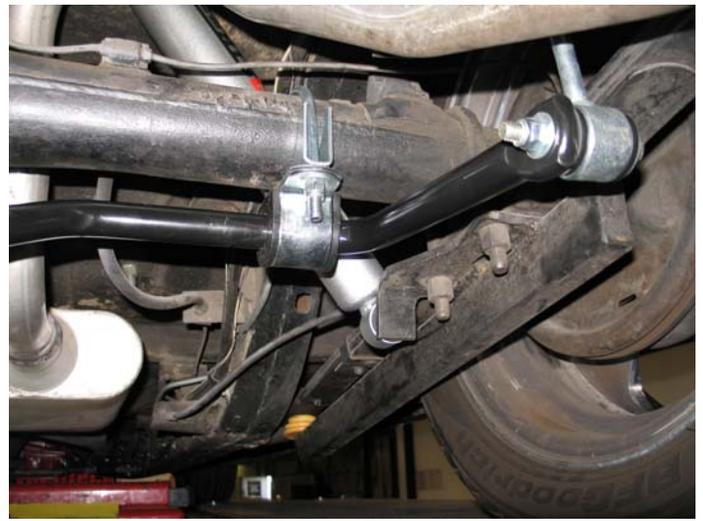
4. Using an existing hole on both side of the frame, measure  $2 \frac{3}{8}$ " from edge of hole to edge of bracket.
