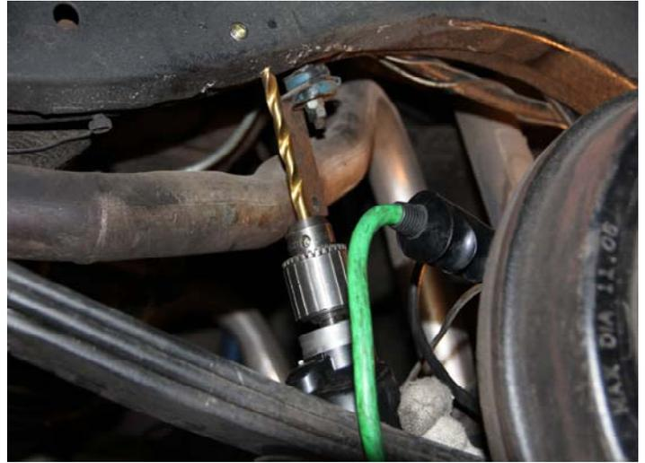
5. You must follow the installation instructions for kit No. 5501 attached when installing these brackets. Holes must be drilled in the correct place. Failure to do this will result in the miss alignment of the bracket.
