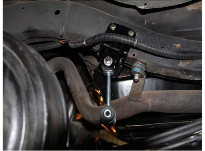
6. After frame brackets have been installed, install the end link to the bracket. Hand tight.
