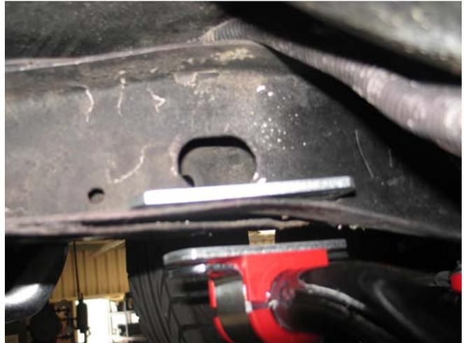
9. After drilling the holes, lubricate the swaybar bushing and reinstall onto swaybar. Using the hardware supplied install the bushing brackets and frame support plates (photo 6) one support plate between the bushing and the frame and the other inside and on top of the frame. Positioning the bolt with a washer on dropping down from inside the frame is easier. Attach bracket and then tighten all hardware.
