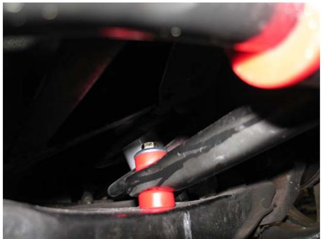
8. With the end links located, install the bushing and bushing brackets without lubrication and position them directly under the frame. Mark the position of the four mounting holes. Center punch the hole locations and drill four 3/8" diameter holes. (photo 5)
