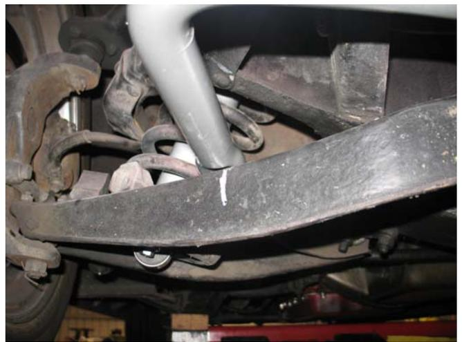
7. After drilling the holes, assemble the end links so the sway bar is in the correct position. (photo 4)
