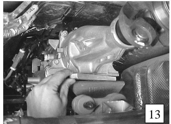
**For applications with a two-piece driveline** and center-carrier bearing you will need to use the supplied transmission spacer and re-locate the center carrier bearing mount.
