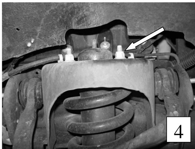
2e) Remove the top three mount bolts of the front spring/strut assembly. **(photo 4)** Slide the spring and shock assembly down and out of the front suspension. For ease of reinstallation, mark the outboard side of the spring and upper shock mount with a paint pen.
