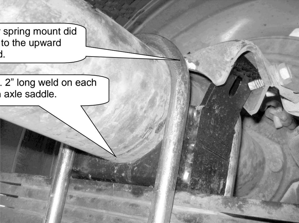
This factory spring mount did not hold up to the upward applied load.
