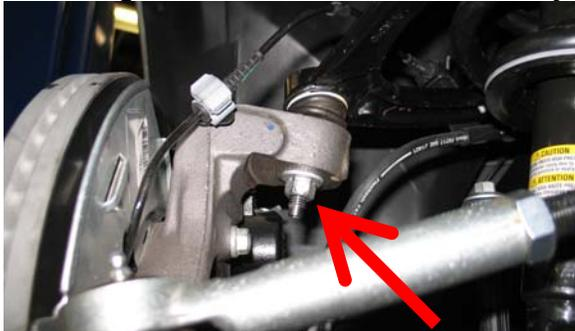
6c. Reattach the swaybar end links to 18ft-lbs.
