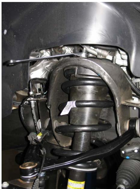
2c. As you did for the top mounts, remove the two bottom mounting nuts of the spring/strut assembly.
