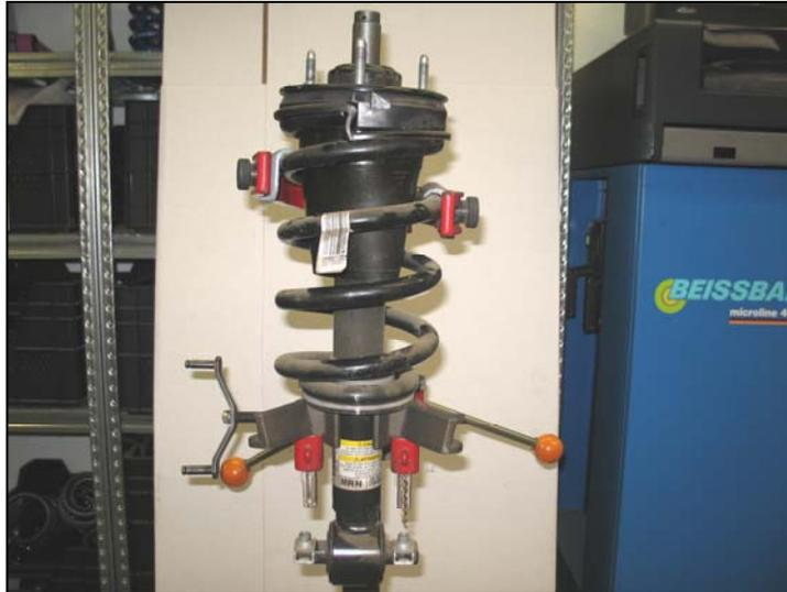
5b. Using an 18mm socket wrench, remove the top mount.
