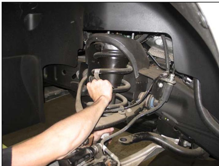
**!** Coil springs may be under tension. Springs under tension store a great amount of energy. Use caution during the following steps to avoid personal injury and/or damage to vehicle. Be careful not to damage the brake hoses.
