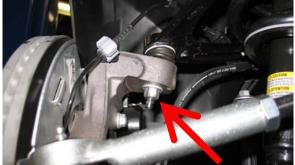
6c. Reattach the swaybar end links to 18ft-lbs.
