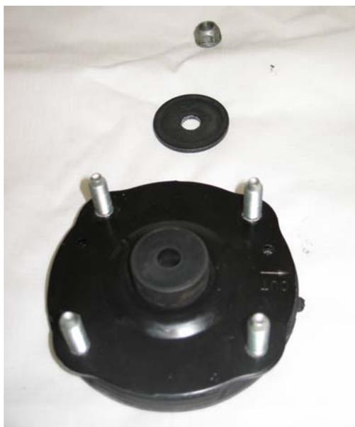
5d. Install your required spacers for the desired height onto the BELLTECH shock. (page 6)
