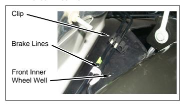
**c.** Remove bolts attaching brake line brackets from driver side.
