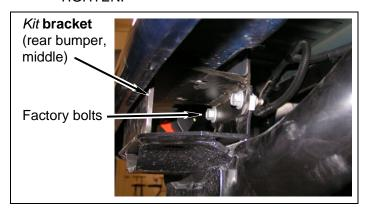
**b.** Apply a few drops of *kit* **Loctite**® to factory bolts. Install *kit* **brackets** (rear bumper) to frame with factory hardware. DO NOT TIGHTEN.
