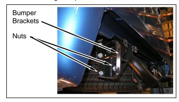
**h. 2003-2004 Models**: Remove two nuts and bolts attaching bumper brackets to trailer hitch.
