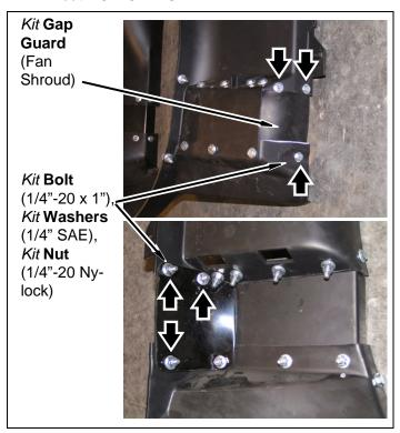
**I.** Ensure a 3" spacing between upper and lower portions of fan shroud. Tighten all hardware.
