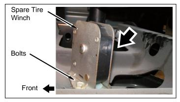
b. Install kit bracket (spare tire winch) on crossmember and locate with factory driver side bolt.
