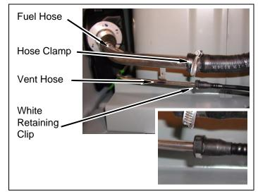
**b.** Remove hose clamp and fuel hose, vent hose and fuel filler assembly from vehicle.
