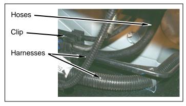
h. Automatic transmission models: Remove transmission wire harness from frame mount clip.
