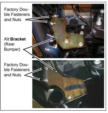
d. Install rear bumper to kit bracket (rear bumper, middle) with two kit bolts (7/16" x 1-1/2"), four kit washers (7/16" USS) and two kit nuts (7/16" Nylock). DO NOT TIGHTEN.
