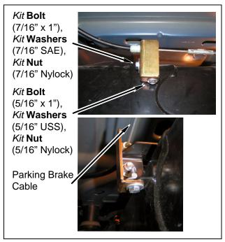
**d.** Route front parking brake cable through largest hole in *kit* **bracket** (parking brake) and connect parking brake cable.
