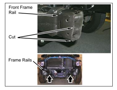
**b. 1500 Models:** Trim lower edges of driver and passenger front bumper brackets.
