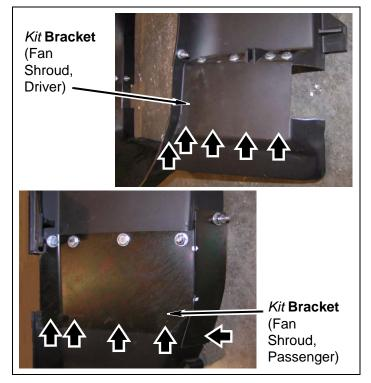
i. Attach kit brackets (fan shroud) to lower portion of fan shroud with kit bolt (1/4"-20 x 1"), two kit washers (1/4" SAE) and kit nut (1/4"-20 Nylock) at each drilled hole location. Snug, but DO NOT TIGHTEN.
