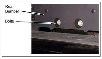
**e.** Remove four nuts and double bolt fasteners attaching bumper to bumper brackets.
