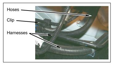
c. Install clip on driver side frame, if possible.
