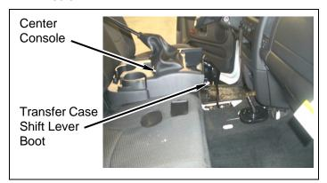
**f.** Remove six bolts attaching shift lever boot seal to floor.
