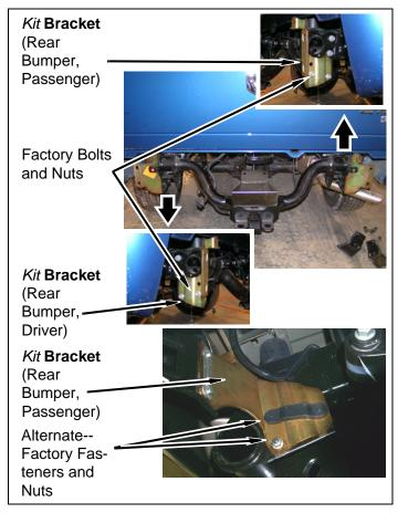
c. Apply a few drops of kit Loctite® to factory bolts. Install rear bumper on kit brackets (rear bumper) with factory two double bolt fasteners and four nuts. DO NOT TIGHTEN.
