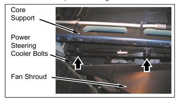
n. Position fan shroud onto radiator. Ensure fan shroud tabs are seated completely in radiator slots. Install fan shroud to radiator with two factory bolts.
