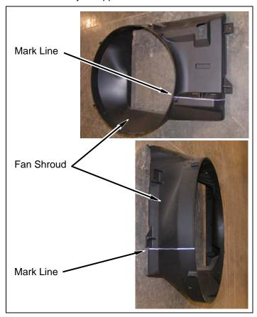
**b.** Cut fan shroud along marked lines in two halves.
