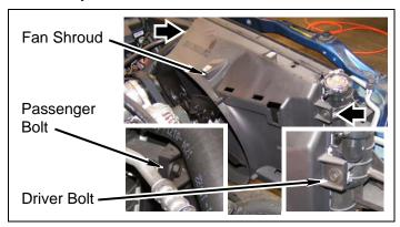
**o.** Pull fan towards radiator off fan clutch shaft. Install bolts securing fan to fan clutch.
