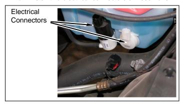
**c.** Install bolts securing radiator overflow and window washer reservoirs to fan shroud.
