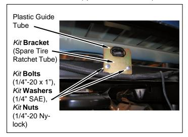
i. Install ratchet tube on spare tire winch with retaining clip.
