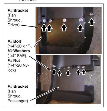
**g.** Position lower portion of fan shroud with *kit* **brackets** (fan shroud) 3" from upper portion of fan shroud as shown.
