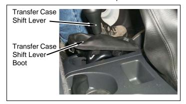
**c.** Unscrew transmission shift lever from shift tower.
