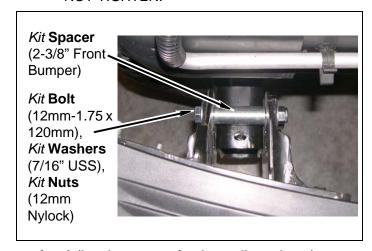
**k.** Adjust bumper to fender until previous bumperto-fender measurement is obtained. TIGHTEN bolts.  Connect fog light harness at driver side of front bumper and install onto front bumper, if equipped.
