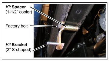
c. Install power steering cooler on two kit brackets (2" S-shaped) with two kit washers (1/4" SAE) and two kit nuts (1/4"-20 Nylock). DO NOT TIGHTEN.
