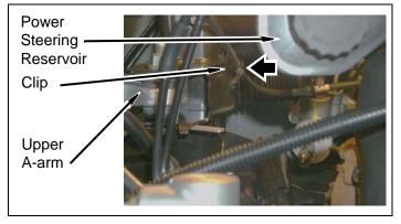
b. 2003-2004 Models: Remove brake lines from retaining clip on driver and passenger front inner fender wheel well.
