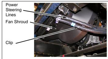
**c.** Remove two bolts attaching fan shroud to radiator.
