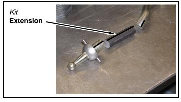
**c.** Grind welded surfaces smooth in order to install mounting plate and shim to shift lever.
