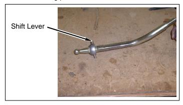
**d.** Install two plastic shift tabs, plastic ball, shim and mounting plate on shift lever.
