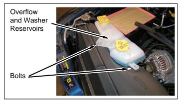
**b.** Disconnect and cap off overflow and washer hoses.
