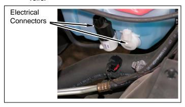
**d.** Remove radiator overflow and window washer reservoirs from fan shroud.
