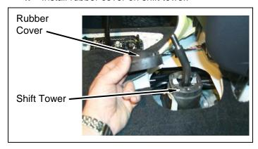
**g.** Install shift lever boot seal to floor with six bolts.
