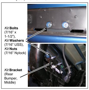
**e.** Install *kit* **brackets** (rear bumper) to bumper with two factory bolts and nuts. DO NOT TIGHTEN.
