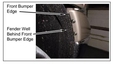
h. Install front bumper and four kit brackets (front bumper) with two factory double bolt fasteners and four nuts. Snug hardware, but DO NOT TIGHTEN.
