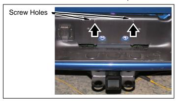
**c.** Remove two bolts attaching bumper bracket to bed.
