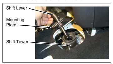
**j.** Remove two plastic shift tabs, plastic ball, shim and mounting plate from shift lever.
