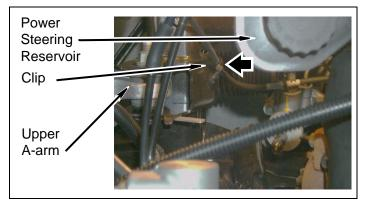
d. 2003-2004 Models: If possible, install brake lines on retaining clip on driver and passenger front inner fender wheel well.
