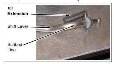
b. Scribe a line along side of kit extension (manual transmission shift lever). Position kit extension between two pieces of transmission shift lever. Ensure scribed lines on kit extension and transmission shift lever align. Weld kit extension in place.
