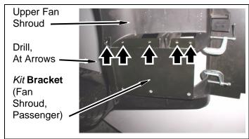
e. Position kit bracket (fan shroud, driver) on outside upper fan shroud. Using kit bracket (fan shroud, driver) as a template, mark and drill a 1/4" hole corresponding to each hole on kit bracket (fan shroud, driver). DO NOT DRILL lower portion of fan shroud at this time.
