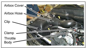
**b.** Remove airbox cover and hose from vehicle.
