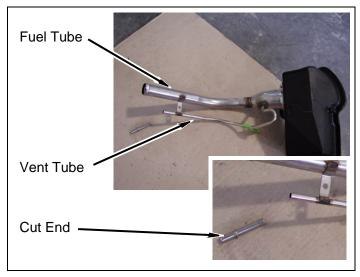
**d.** Install *kit* **extension** (vent, 1/4" x 3") between cut ends of metal vent tube with two *kit* **clamps** (#6 hose). DO NOT TIGHTEN.
