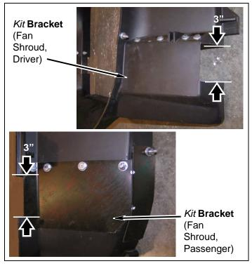
**h.** Using *kit* **brackets** (fan shroud) as templates, mark and drill a 1/4" hole corresponding to each hole on *kit* **brackets** (fan shroud).
