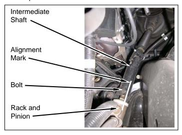
**c.** Remove bolt and intermediate shaft from rack and pinion. Slide intermediate shaft up to separate from rack and pinion.
