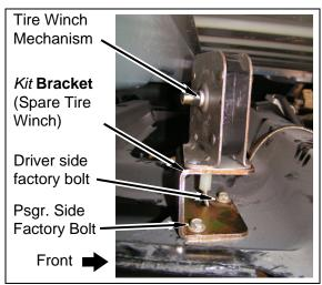
c. Install spare tire winch through hole in crossmember. Install spare tire winch on kit bracket (spare tire winch). **d.** Turn *kit* **bracket** (spare tire winch) toward front of vehicle and slide spare tire winch cable through slot in *kit* **bracket** (spare tire winch).
