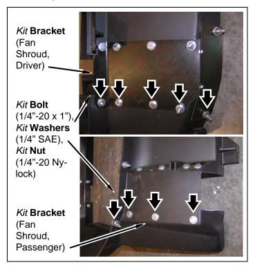
j. Position kit gap guard (fan shroud) inside upper and lower portions of fan shroud. Using kit gap guard (fan shroud) as a template, mark and drill a 1/4" hole corresponding to each hole on kit gap guard (fan shroud).
