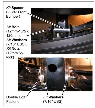
j. 2500 Models: Install two kit spacers (2-3/8" front bumper) between top holes of four kit brackets (front bumper) and factory bumper brackets with two kit bolts (12mm-1.75 x 120mm), four kit washers (7/16" USS) and two kit nuts (12mm Nylock). Snug hardware, but DO NOT TIGHTEN.
