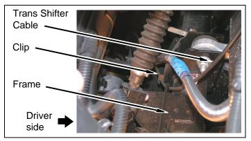
**g. Automatic transmission models:** Remove clip, two harnesses, hose and three hard lines from frame driver side.
