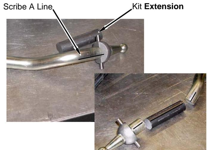
b. Position kit **extension** transmission shift lever 5/8" x 3" between two pieces of transmission shift lever. Ensure kit **extension** and shift lever scribe lines align and weld extension in place. Let shift lever cool.
