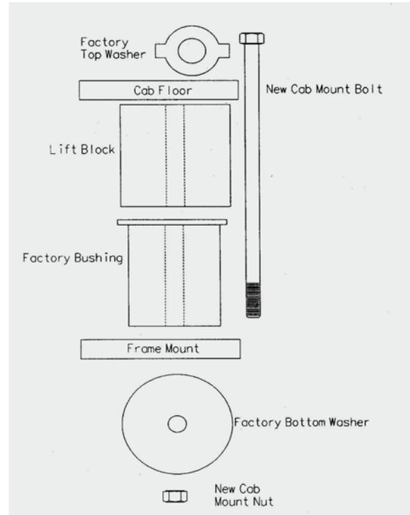
17. Repeat step 16 for the driver's side of the cab. Realign the cab to the bed. Refer to measurements made earlier. Remove the nuts from the body bolts one at a time. Apply Loctite® to the nuts and bolts. Reinstall the nuts on the bolts. Tighten all cab mounting bolts securely.
