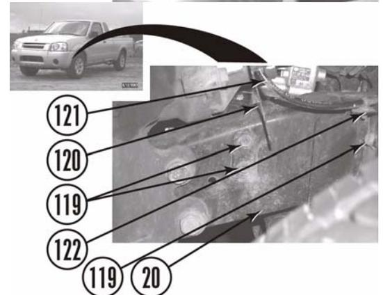
n. Remove bolt (119) and bracket (122) from hose (121) and frame (20) driver side.
