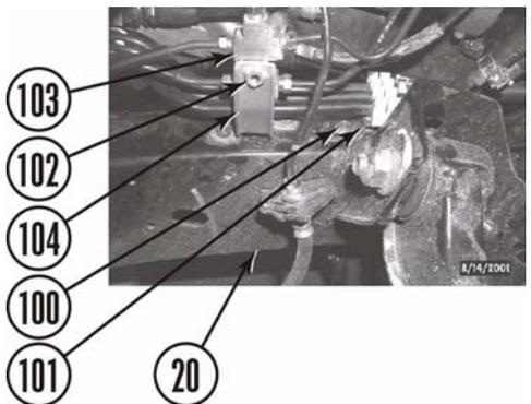
d. Install brake module (103) on bracket (104) with bolt (102).
