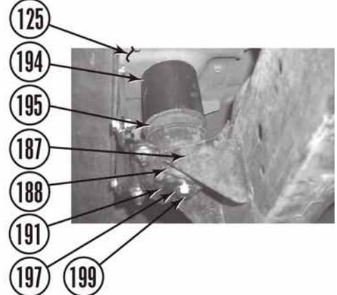
3. Install the cab driver side spacer blocks.
