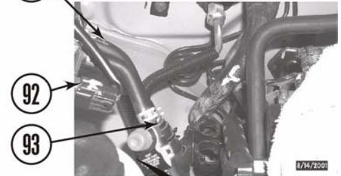
c. Remove wire harness (94) from clip (95) on passenger side wheel well (67) behind power steering reservoir (88).
