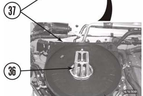
f. Remove vacuum hose (38) from passenger side throttle body (34). Leave vacuum hose connected to lower air cleaner housing (37).
