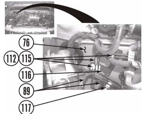
j. Remove two bolts (118) and bracket (116) from fire wall (76).
