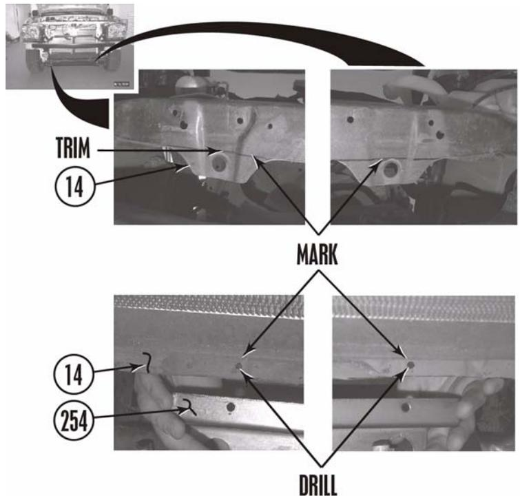
b. Install *kit* lower radiator support bracket (254) on core support (14) with two *kit* 1/4" x 1" bolts (237), four *kit* 1/4" washers (238), and two *kit* 1/4" nylock nuts (239).
