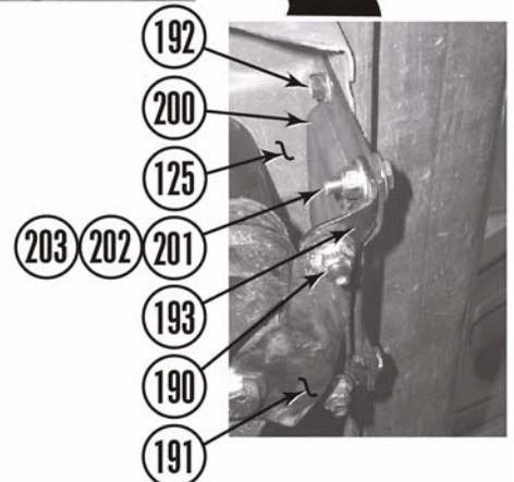
5. Finish cab spacer block installation.
