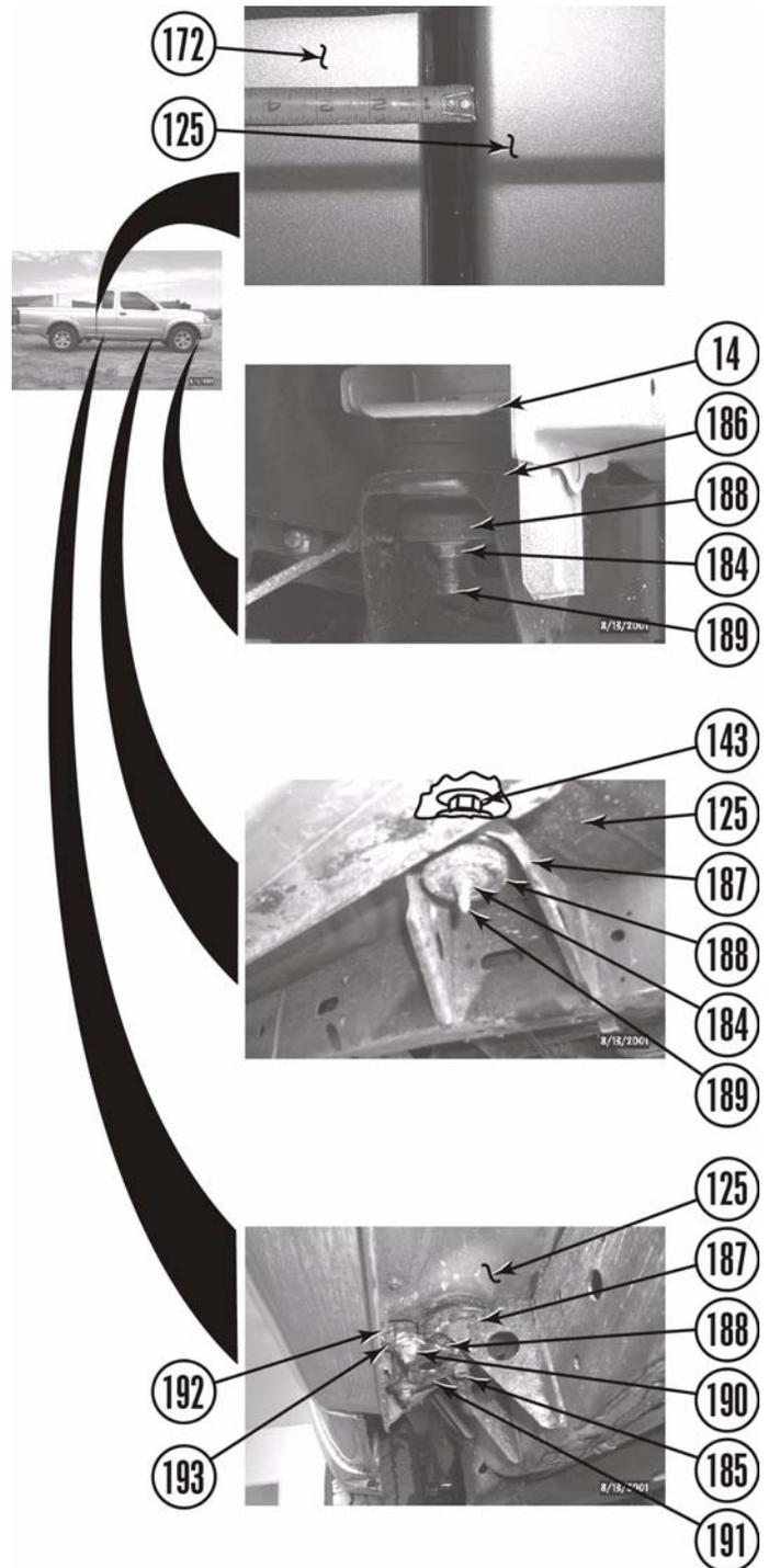
2. Lift cab and install passenger side spacer blocks.
