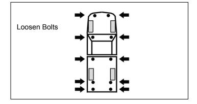
b. Remove body mount bolts from passenger side of vehicle ONLY.
