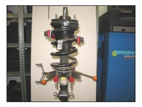
5b. Using an open wrench, remove the top mount.
