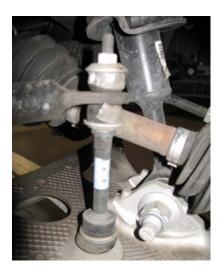
3b. Locate Steering arm link at spindle. Unbolt the steering arm bolt and disconnect stud from spindle.
