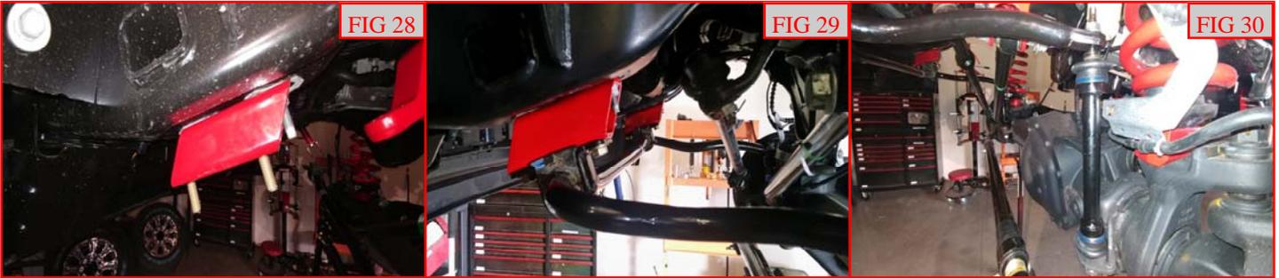
Install the ReadyLIFT® sway bar brackets to the frame using **factory hardware**. Torque to **45 ft-lbs**. Install the factory sway bar to the ReadyLIFT® brackets using **7/16" x 1.5" bolts, washers, and nuts**. Torque to **55 ft-lbs**. Install the ReadyLIFT® sway bar end links to the axle and sway bar using the **supplied nuts**. Torque to **45 ft-lbs**.
