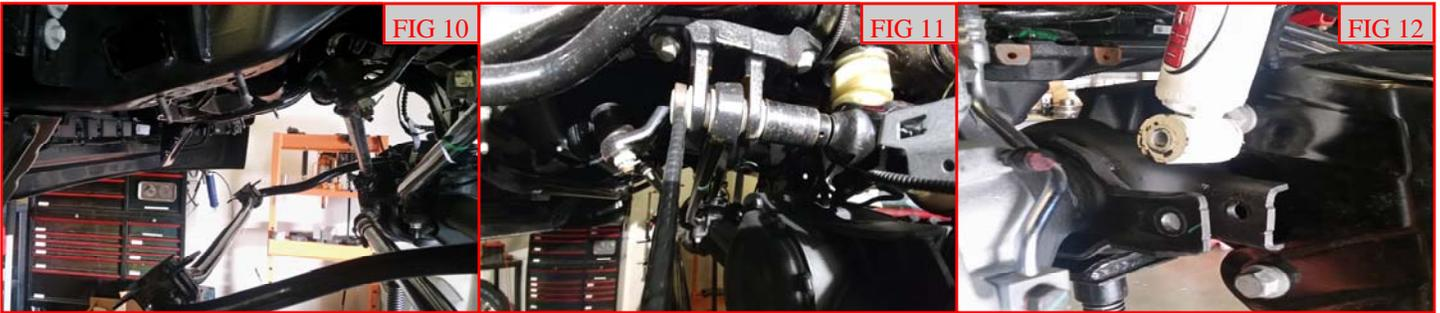
Remove the sway bar from the frame. Note orientation of the bar for re-install. Remove the track bar at the track bar bracket. Remove the shock from the axle. (FIG 10, 11, 12)
