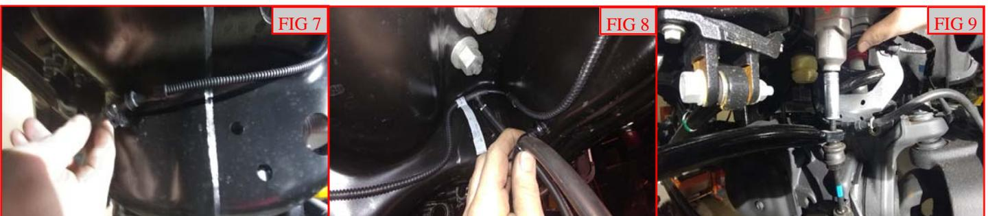
Remove the vacuum line at the 2 points on the engine cross member. Remove the axle vent line tube from the top of the driver side shock and the inside frame rail. Remove the sway bar end links from the sway bar and axle. (FIG 7, 8, 9)
