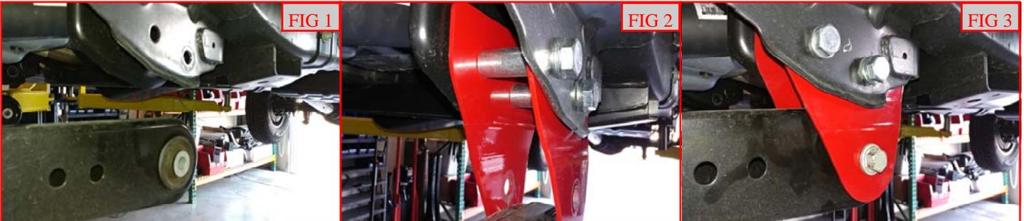
Remove the radius arm at the frame. Rotate the axle until there is enough clearance to install the ReadyLIFT® radius arm drop brackets. Install the ReadyLIFT® radius arm drop brackets into the frame using **M18 x 130mm bolts, washers, crush sleeve, and nuts**. Do not tighten at this time. Rotate the axle until you can line up the radius arms into the ReadyLIFT® drop brackets. Install using **factory hardware**. Do not tighten at this time. (FIG 1, 2, 3)
