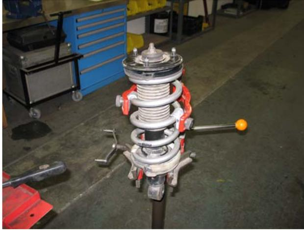
5b. Using a socket wrench, remove the top mount.
