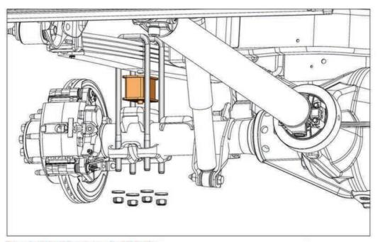
Torque U-bolt hardware to 75 ft. lbs. Never reuse U-bolts
