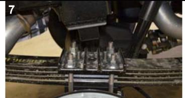
Carefully raise axle and install replacement Traxda U-Bolts. Torque to manufacturers specifications. Reinstall lower shock mount.
