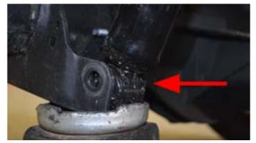
Raise rear of vehicle and support with jackstands at frame on both sides. Remove wheels, support axle on one side and remove the lower shock mounting bolt.
