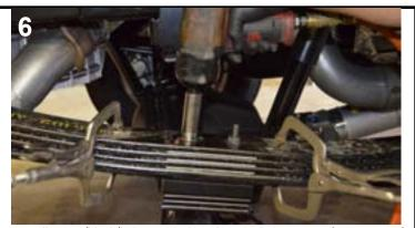
Re-install spring/block/bolts to vehicle and torque bolts to manufacturer specifications. The spring center bolts may need to be trimmed after tightening.
