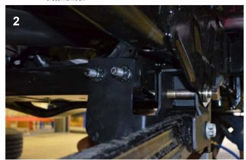
Install radius arm bracket, using supplied bolt and OEM crossmember nuts
