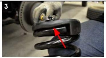
Remove the coil spring and rubber spring isolator from the vehicle.
