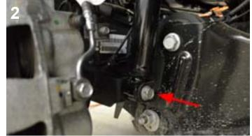
Disconnect the front shock absorbers at the axle mounts on both sides. Carefully lower the front axle using jack until the coil spring is loose.
