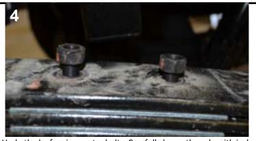
Undo the leaf spring center bolts. Carefully lower the axle with jack.
