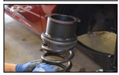
Re-install the isolator onto the spring, and mount the Traxda Coil Spacer above it. Repeat steps 3 and 4 for other side of vehicle.
