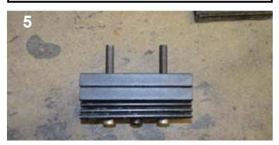
Replace old center bolts with Traxda bolts. Install Traxda lift block as show above. Install two blocks per side, and bolt with center bolts
