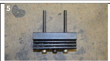
Replace old center bolts with Traxda bolts. Install Traxda lift block as show above.
