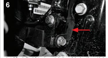
Install Traxda Shock Extensions onto bottom of shocks with provided hardware. Using factory hardware attach extensions onto axle.
