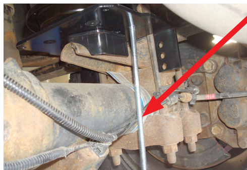
The long carriage bolt goes on the outside (backside) of the hard brake/ABS line on the passenger's side.
