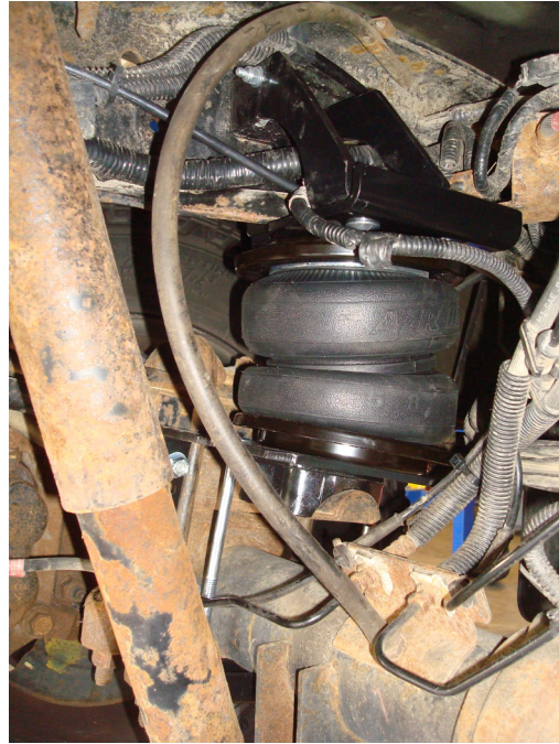
Back center driver's side view of the kit installed.
