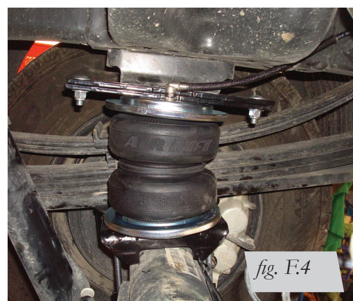
Inside view of the passenger's side installation.
