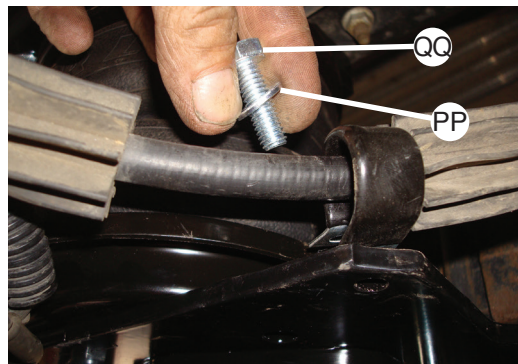
Attach P-clamp to the corner of the lower bracket.
