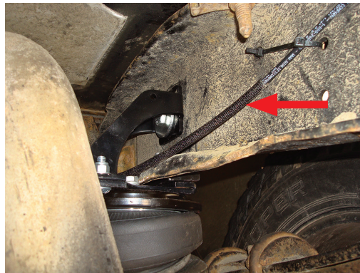
Hose heat shield shown in place on the right side (passenger) of the vehicle. Make sure heat shield is pushed up against the fitting once the hose is installed.
