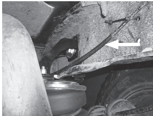
Hose heat shield shown in place on the right side (passenger) of the vehicle. Make sure heat shield is pushed up against the fitting once the hose is installed.
