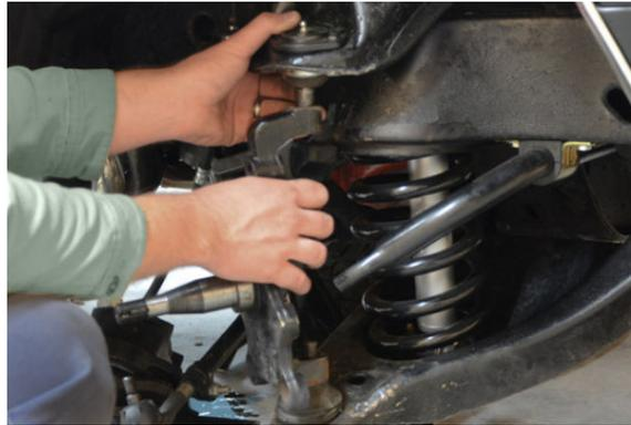
18. The steering arm will attach to the back of the spindle at the bottom holes. The steering arm is thicker on the tie rod end side; use the 1/2"-20 X 2-1/2" bolt on the tie rod end side bolt hole and the 1/2"-20 X 1-3/4" bolt on the opposite end. Place the bolts with the bolt head on the rotor side and the threaded shaft through the back of the spindle. Fasten the bolts with 1/2"-20 Nyloc nuts and torque to 85 ft lbs.
