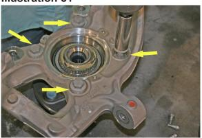
□ [Illustration 52] Install the new knuckle (66-01-9930 driver's side and 66-02-9930 passenger's side) onto the hub bearing assembly. Apply thread locker to the factory hardware and install bolts; tighten. (151) {18mm}
