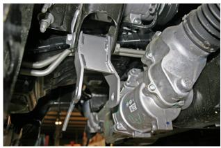
□□ [Illustrations 35 & 36] Position the front driver differential bracket into the frame using the factory hardware; install bolt from front, then pivot the differential into the passenger side differential bracket and secure using the supplied 9/16" x 3-3/4" bolts, washer, and nut; install bolt from rear. Do not tighten.
