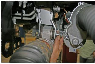
☐ [Illustration 37] Attach the hose adapter to the new vacuum hose, then attach the hose adapter to the factory hose. Connect the new hose to the differential.
