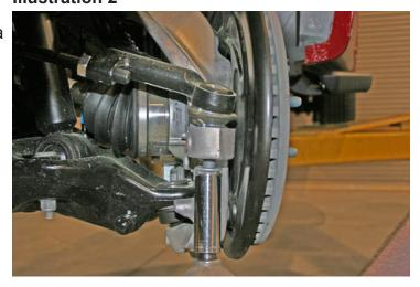
□□ [Illustration 4] Remove the ABS sensor wire from the steering knuckle. {8mm}
