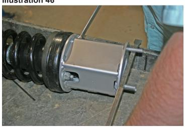
□□ [Illustration 49] Tighten the three top strut spacer 10mm flange nuts. (55) {15mm}
