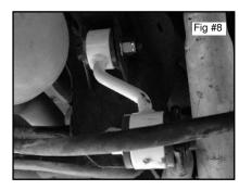
Apply some grease to the bushing and bolt the passenger side end link to the factory upper mount using factory hardware. The lower end is offset to the passenger side. Bolt the sway bar to the outside of the end link using 1/2" x 2-3/4" bolts (Fig # 8)
