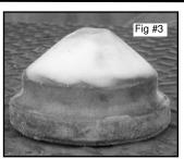
Remove factory orange bump stop and cut off first ring. To give the bump stop a more custom look we modified it on our belt sander. Reinstall bump stop.
