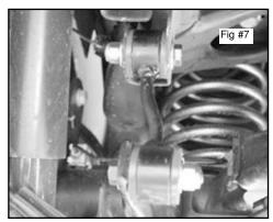
Apply some grease to the bushing and bolt the driver side end link to the factory upper mount using factory hardware. The lower end is offset to the passenger side. Bolt the sway bar to the outside of the end link using 1/2" x 2-3/4" bolts (Fig # 7).
