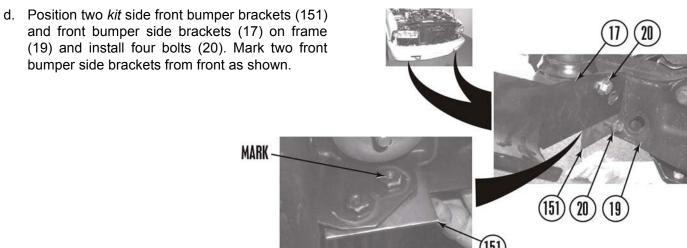
e. Remove two front bumper side brackets (17) and drill where marked using 13/32" drill bit.
