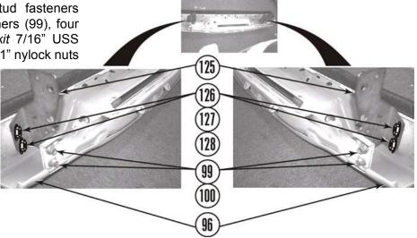
d. Loosely position two kit rear bumper brackets (125) and rear bumper (96) on frame (19) and install two license plate lights (82), three clamps (103) and harness (104) on rear bumper.
