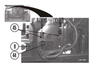
b. Install positive battery cable box (43) on bracket (44).
