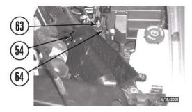
m. Install air filter (62) in air filter housing (54). Install air filter housing cover (53) on air filter housing with four screws (52).
