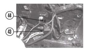
c. Drill two 13/32" holes in wheel well (49) 1/2" toward center of vehicle from old holes as shown.
