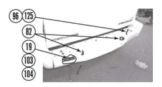
e. Install two *kit* rear bumper brackets (125) on frame (19) with two double stud fasteners (100), four nuts with captive washers (99), four *kit* 7/16" x 1 1/2" bolts (129), eight *kit* 7/16" USS washers (127), and four *kit* 7/16" nylock nuts (128). Do not tighten.
