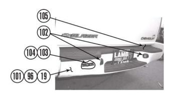
f. Remove four nuts with captive washers (99), two doubles stud fasteners (100), four bolts (106), and two rear bumper brackets (101) from rear bumper (96).
