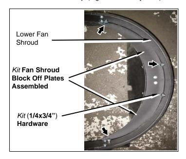
k. Install kit lower fan shroud block off plate anchor onto kit lower fan shroud block off plate assembly by using existing kit (1/4") hardware and drilling a 1/4" hole into center of the shroud and installing kit (1/4") hardware to anchor center of lower shroud assembly.
