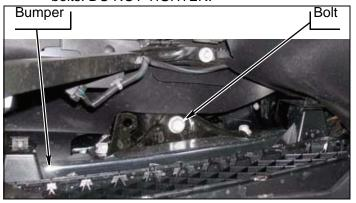
g. Install two kit brackets (bumper, front, support) onto bumper with two kit large washers between bumper and kit bracket. DO NOT TIGHTEN
