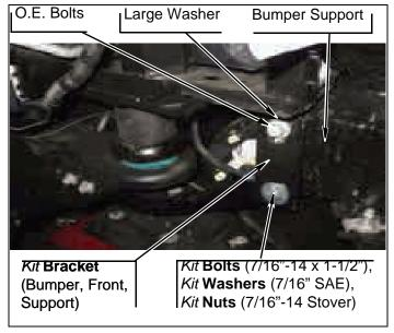
i. Adjust bumper to body clearance using measurements from removal section. Align bumper to previous measurements and TIGHTEN all bumper hardware.
