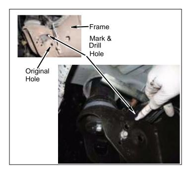
b. Relocate parking brake cable into *kit* **park bracket** and mount using *kit* **7/16**" hardware. .
