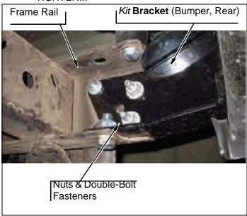
q. Install kit **bracket**, hitch spacer, on rear bumper and hitch with two kit **bolts** (14mm x 110mm) and two kit **washers** (14mm). Do not tighten.
