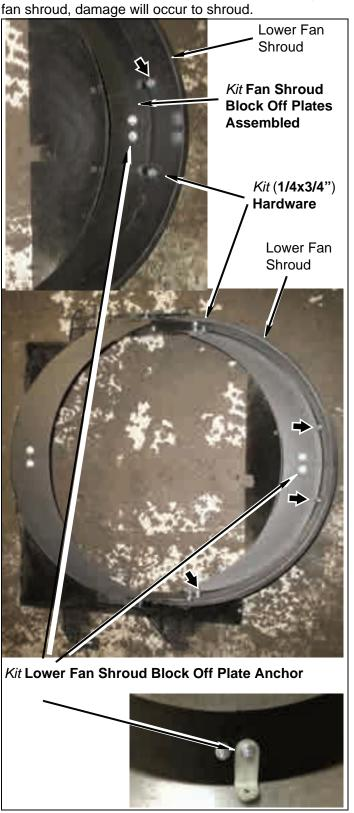
I. Install engine fan and shroud assembly as one unit; use a fan clutch tool to tighten fan clutch. .
