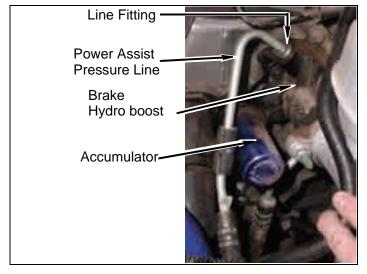
g. Remove bolt, clamp, and power assist pressure line from frame.
