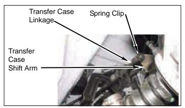
Scribe a line along transfer case linkage as shown. Cut transfer case linkage into two pieces through the scribed line and deburr.
