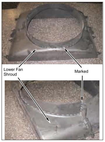
b. Trim cut along marked line and remove lower section of lower fan shroud.
