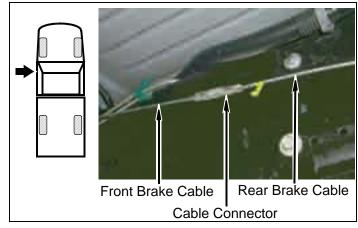
Remove front bake cable and brake cable housing from front frame mounting pad.
