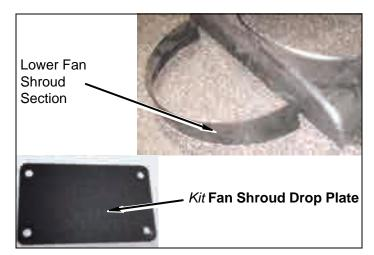
c. Using a pair of visegrips or clamps; create a 3" gap at the center of the fan shroud by separating & squaring the main engine fan shroud with the lower fan shroud insert shield; then clamp the assembly together using two kit side shroud drop plates at each side.
