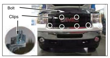
Install cover on core support with seven push pins.
