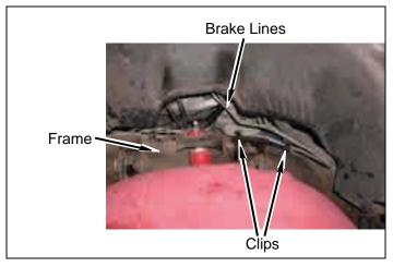
c. If possible, install harness in clip on frame driver side.
