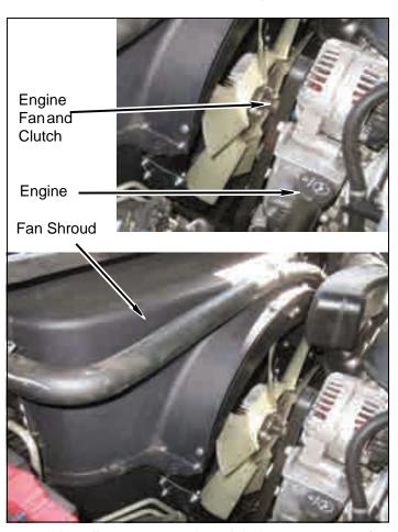
m. Install two upper shroud bolts onto upper fan shroud and core support.
