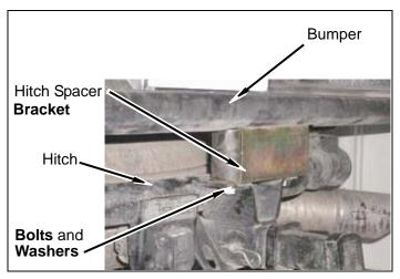
r. Adjust bumper to bed clearance using measurements taken earlier and tighten hitch bolts first then remaining bolts and nuts to 55 lbft. s. Plug license plate light harness in at crossmember connector.
