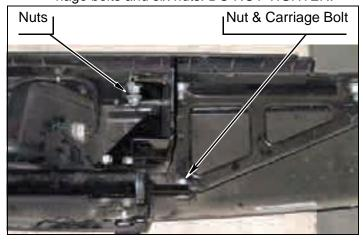
Install bottom of bumper onto bumper support with two bolts.
