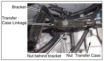
Remove two clips and transfer case linkage from transfer case and pivot.
