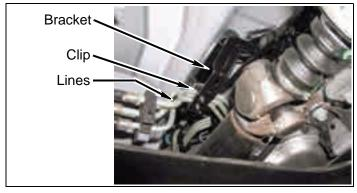
b. Remove two nuts and bracket from transfer case. Bracket is not reused. Install two nuts and tighten.
