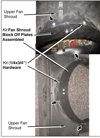
Using second pair of kit fan shroud block of plates. (Leave brackets slightly loose until mounted onto fan shroud, this will allow you to adjust the plates as needed to fit shroud properly.) With both kit fan shroud block off plates assembled, face the tabs outwards so that the kit fan shroud block off plate assembly mounts evenly with the inside edge of the lower fan shroud assembly. (Tighten assembly now.)
