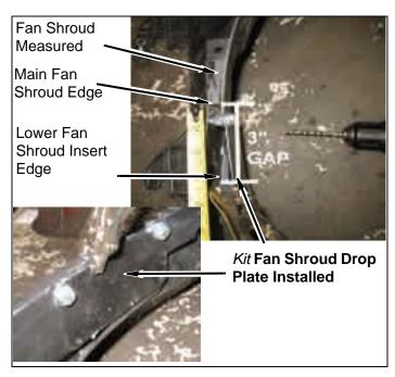
d. Once you have shaped and placed each kit fan shroud drop plates into place; reclamp and secure each kit shroud plate at a 3" gap and mark each 1/4" holes for drilling.
