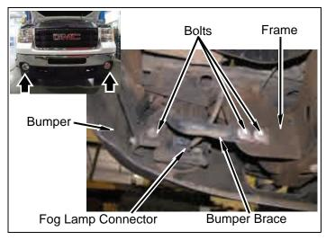
c. Remove two bolts from each fender side and remove bumper face from core support and fenders.
