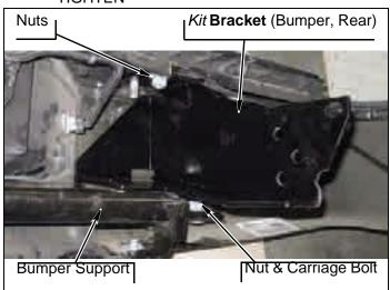
**g.** Install bumper onto frame rails with all O.E. double-bolt fasteners. Snug, but DO NOT TIGHTEN.
