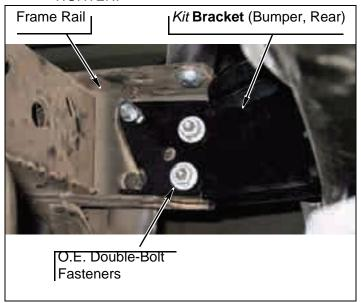
**h.** Mark eight holes through two *kit* **brackets** (bumper, rear) onto bumper support.
