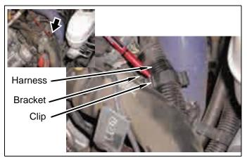
c. Remove two clips and harness from cover and inner fender.
