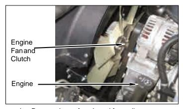
d. .Remove lower fan shroud from clips.
