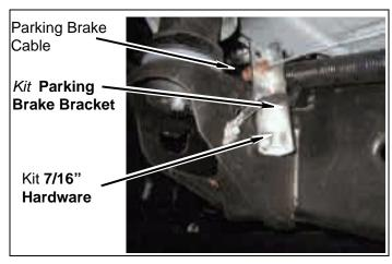
c. Install two ground wires on frame mounting pad with bolt. Connect front and rear brake cables. Remove clamps from rear cable. Note: Kit washer may be used between kit bracket and body mount to keep bracket aligned.
