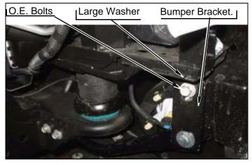
h. Install two bumper supports onto kit brackets with two kit bolts (7/16"-14 x 1-1/2"), four kit washers (7/16" SAE), two kit nuts (7/16"-14 Stover) with four O.E. bolts to body mount. DO NOT TIGHTEN.
