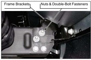
Remove four bolts, two nuts and two tow hooks from frame horns.
