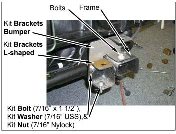
d. 2" kit: Install two kit brackets bumper and two kit brackets C-shaped on frame with two stock bolts, two kit bolts (7/16" x 1 1/2"), four kit washers (7/16" USS), and two kit nuts (7/16" nylock). Do not tighten.
