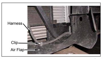
e. Remove two clips, three push pins, and air flap from core support.
