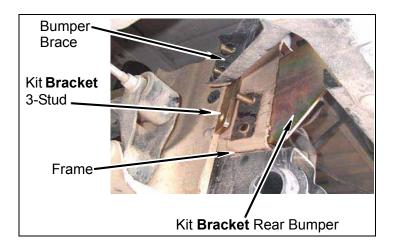
g. **3" kit passenger side:** Install kit **bracket** (3-stud) on outer bumper brace with two kit **washers** (1/2" USS), and two kit **nuts** (1/2" nylock), on two studs as shown. Do not tighten
