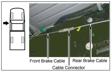
d. Remove front bake cable and brake cable housing from front frame mounting pad.
