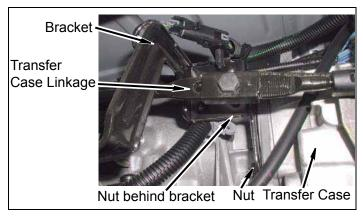
c. Remove two clips and transfer case linkage from transfer case and pivot.
