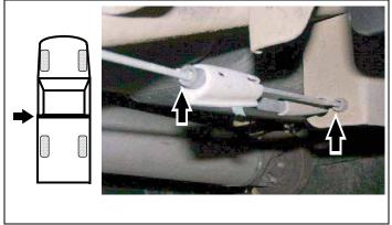
c. Separate front parking brake cable from rear parking brake cable at cable connector.
