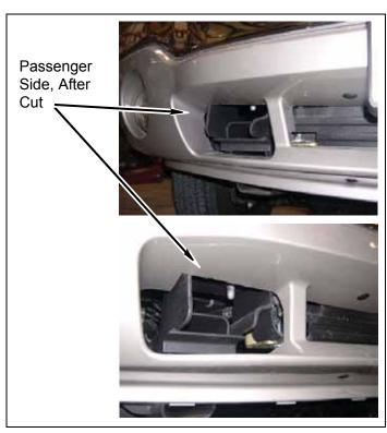
h. Install front bumper on kit **brackets** bumper and with four kit **bolts** (7/16" x 1 1/2"), eight kit **washers** (7/16" USS), and four kit **nuts** (7/16" nylock). Do not tighten.
