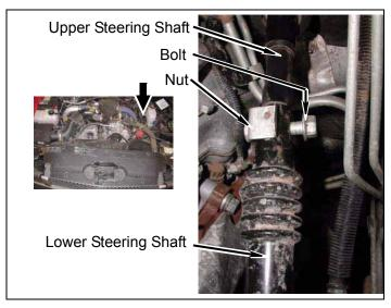
c. Slide upper steering shaft up to separate from lower steering shaft.
