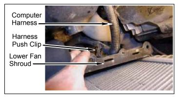
e. Lift lower fan shroud from radiator clips on side of radiator body.
