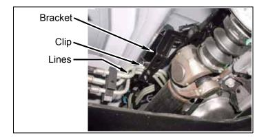
b. Remove two nuts and bracket from transfer case. <u>Bracket is not reused.</u> Install two nuts and tighten.
