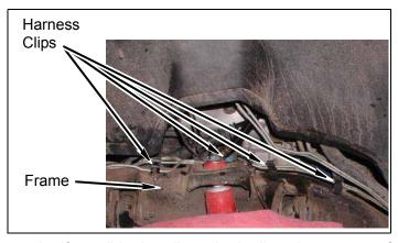
d. If possible, install two brake lines in two sets of clips. If brake lines will not fit back into position, wrap lines with two kit **zip ties** individually, and then secure the lines together with one kit **zip tie** as a bundle.
