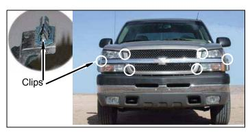
b. Install cover on core support with seven push pins.
