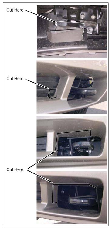
g. GMC models: Repeat above step for passenger side front bumper. Check fitment and trim driver and passenger side, if necessary.
