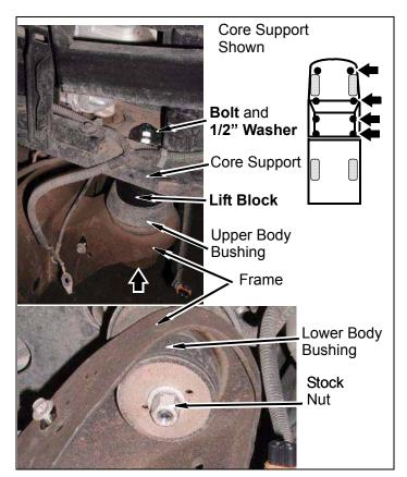
c. Install three kit lift **blocks** (with 5/8" hole) under body and on top of top body bushings, frame, and lower bushings, with three kit **bolts** (14mm-2.0 x 180mm) and kit **washers** (14 mm). Do not tighten.
