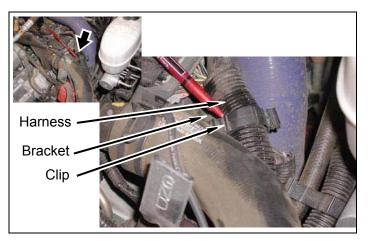
c. Remove two clips and harness from cover and inner fender.
