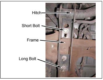
d. Remove two bolts and bumper from hitch and vehicle.
