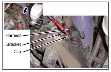
b. Install ground strap on stud with nut.
