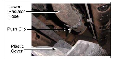
Outline transmission cooler hose on lower fan shroud as shown. (looking up from under vehicle)
