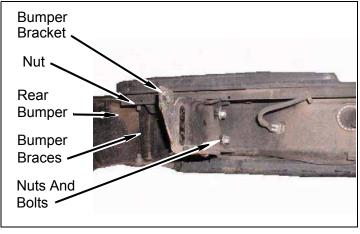
d. Install two kit **brackets** (rear bumper) on rear bumper with four bolts and nuts. Do not tighten.
