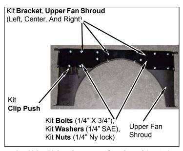
Using kit bracket, upper fan shroud (center) as template, drill two 1/4" holes in fan shroud lip. Install kit bracket, upper fan shroud (center) on upper fan shroud lip with two kit clips push.
