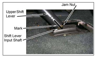
c. Loosen jam nut and remove upper shift lever from shift lever input shaft.
