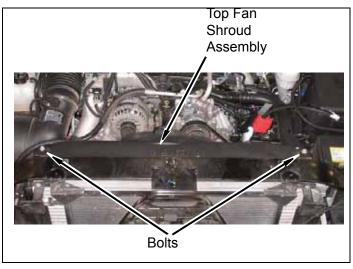
e. Install top fan shroud on bottom fan shroud with four pop-ups. Check fan to shroud clearance. Ensure gap is the same all around shroud.
