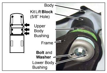
d. Lower cab onto kit lift blocks.
