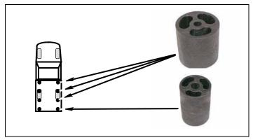
c. Install kit lift **blocks** on frame and bed with four kit **bolts** (12mm-1.75 x 100mm) and four kit **washers** (7/16" USS). Do not tighten.
