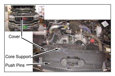
b. Remove bolt, six clips, and grille from core support. Some GMC models may have extra clips.
