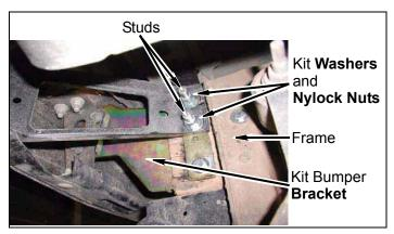
h. **3" kit passenger side:** Install kit **bracket** (3-stud), outer bumper brace, and kit **bracket** (rear bumper) on frame with a kit **bolt** (1/2" X 1 1/2") three kit **washers** (1/2" USS), and two kit **nuts** (1/2" nylock). Do not tighten.
