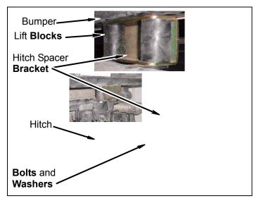
m. Install hitch on frame with two short bolts and nuts. Use forward most hole in hitch.
