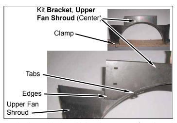
d. Assemble three kit brackets, upper fan shroud (left, center, and right) with two kit bolts (1/4" x 3/4"), four kit washers (1/4" SAE), and two kit nuts (1/4" nylock) as shown. Snug, bolts but do not tighten.
