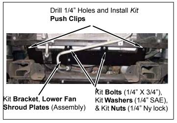
Install Air Flap with three push pins in holes provided in kit lower fan shroud plates. Install two outer Air Flap clips.
