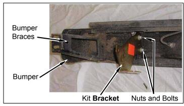
e. Install bumper and kit **brackets** (rear bumper) in frame rails. Ensure spare tire crank tube is possioned in original hole in bumper.
