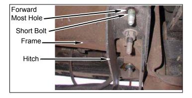
n. Install kit brackets (rear bumper) and hitch on frame with two long bolts, two kit washers (1-1/2 x 2-1/2 rectangular), two kit washers (14mm), into two kit nuts (14mm nylock).
