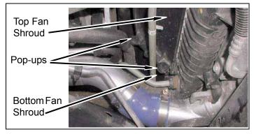
f. Install computer module on upper fan shroud with one pop-up.
