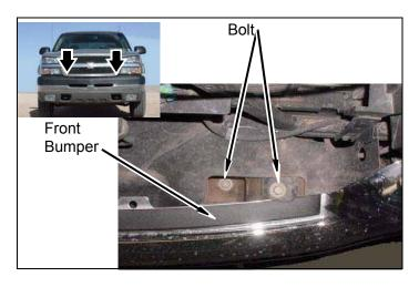
d. Remove six bolts, and two tow hooks from frame.
