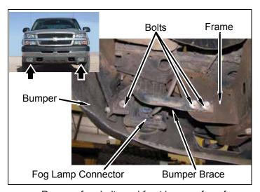
c. Remove four bolts and front bumper from frame.
