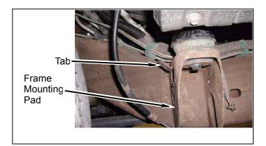
c. Install the front parking brake cable housing as shown.
