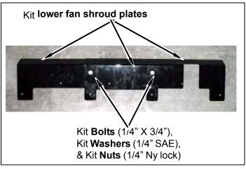
h. Install *kit* **lower fan shroud plates** (assembly) on core support with two kit **bolts** (1/4" x 3/4"), four kit **washers** (1/4" SAE), and two kit **nuts** (1/4" nylock). Using fan shroud plates as template, mark and drill two 1/4" holes in core support as shown. Install two kit push clips in the drilled holes.
