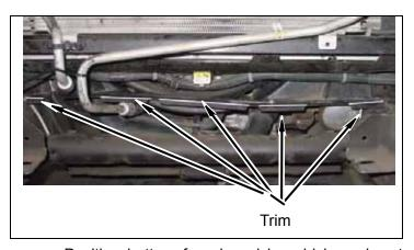
c. Position bottom fan shroud in vehicle and rest below lower core support.
