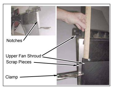
g. Using three kit brackets, upper fan shroud (left, center, and right) as templates, drill 1/4" holes in fan shroud. h. Install three kit **brackets**, **upper fan shroud** (left, center, and right) on upper fan shroud with one kit **clips push**, fifteen kit **bolts** (1/4" x 3/4"), thirty kit **washers** (1/4" SAE), and fifteen kit **nuts** (1/4" Nylock).
