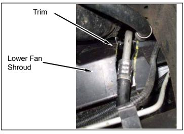
b. Remove bottom lip from lower fan shroud in five places as shown.
