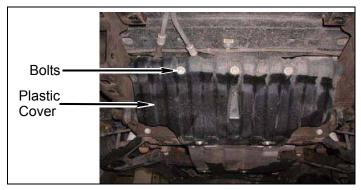
Remove plastic cover from push clip, lower radiator hose and vehicle.
