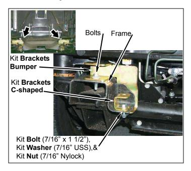
e. Mark and cut two front bumper brackets. Bend bottom edge of bumper bracket up toward bumper.
