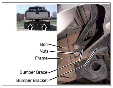
c. If equipped with a trailer hitch, remove two short and two long bolts from hitch and frame.
