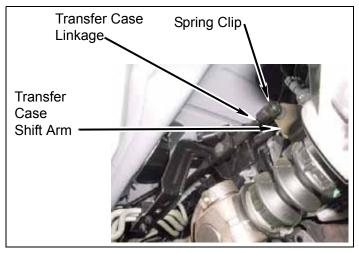
b. Scribe a line along transfer case linkage as shown. Cut transfer case linkage into two pieces through the scribed line and deburr.
