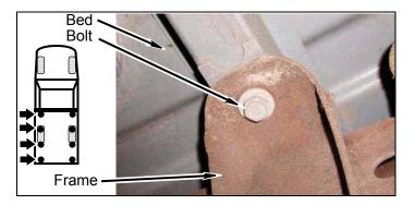
b. Remove four bed bolts from frame passenger side.
