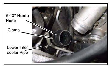
c. Place factory clamp on hump hose. Install factory elbow on intake housing and rotate factory elbow into the *kit* **3" Hump Hose**.
