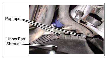
Remove computer wiring harness from harness push clip and lower fan shroud.
